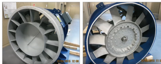
Figure 5: Design of the new 75 kW electric ventilator; left side: stator region after the ventilator rotor; right side: rotor and electric unit.
