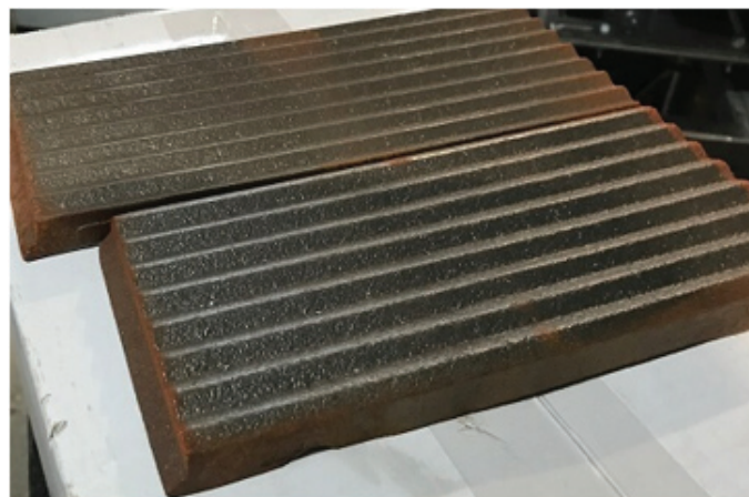
Figure 1: Chilled steel composite stone crusher jaw fabricated for a stone crushing machine.
